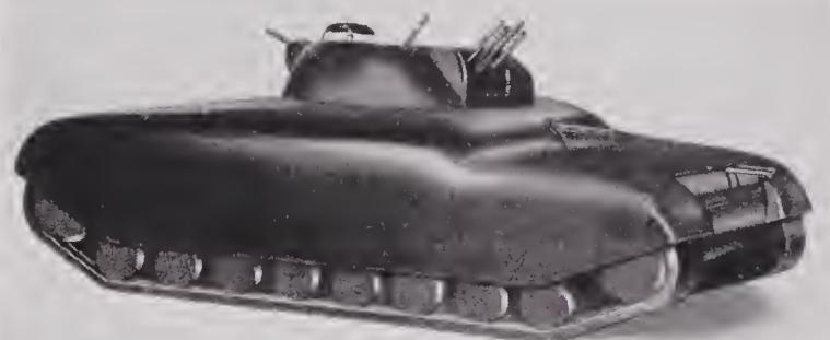
FIGURE 3. Model of IVI-C medium tank equipped with four .50-caliber machine guns.
